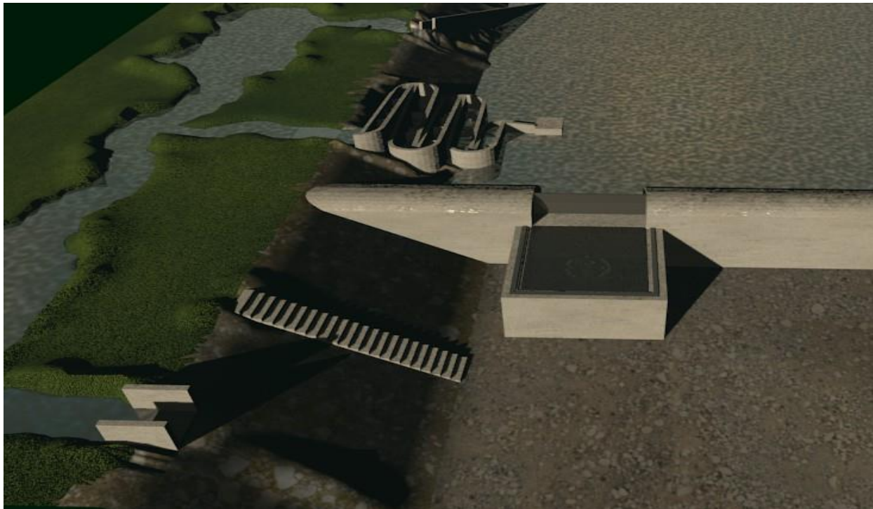
Figure 1: Computer visualization of a classical TUM-HSPP originally intended for energy production at existing weirs (courtesy J. Frank).
